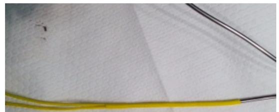
Last you will put a 3 or 4" piece of shrink sleeve over the end of the tubes and the transition tubes. A bit of epoxy under the shrink sleeve will protect the fiber joint.
