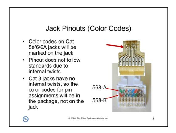
Pinout on Cat 5e/6 jacks will be marked on the back at the punchdowns with the correct color codes
