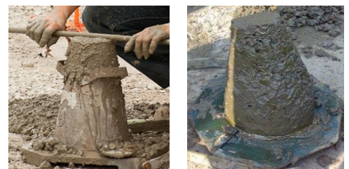
Concrete Slump Test Must not collapse or shear off laterally
