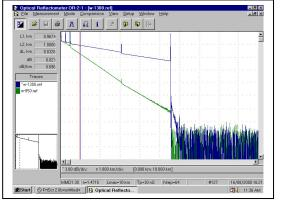
The final parameter is the number of averages for each trace. To improve the signal to noise ratio of the trace, the OTDR can average multiple measurements, but more averaging takes more time. Usually 16-64 averages are adequate.
