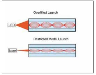
launch cable, including the stiffness of the jacket and amount of strength member fill in the cable. A reputed more consistent method, using mode conditioning patch cords, is now being used in Europe and is now becoming available in the USA.
