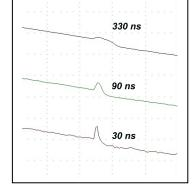
Next choose the wavelength. Normally you start with 850 nm on multimode fiber and 1310 nm on singlemode, since the shorter wavelength has more backscatter so the trace will be less noisy. After initial tests, you can make measurements at the longer wavelengths (1300 nm on multimode and 1550 nm on singlemode) and compare traces
