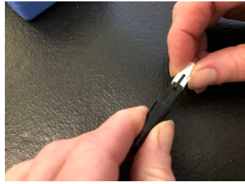
Slide black connector body over heat shring tubing, align groove in body to black line on SOC
