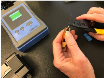
Make sure 250 micron buffer is stripped
