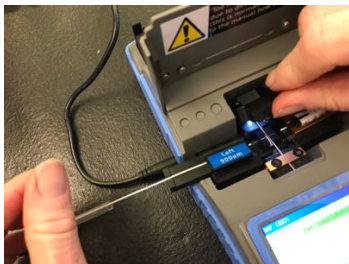
Open lid, lift center bracket
