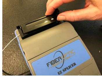
Close oven - Right clamp will not close
