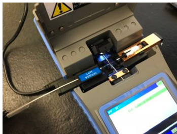
Lift left fiber holder lid carefully
