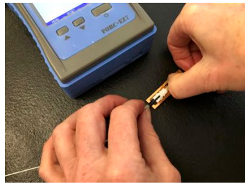
Use fingernail to release SOC and lift out of holder with heat shrink tubing
