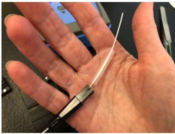
Slip conn body and heat shrink sleeve on fiber to splice to SOC
