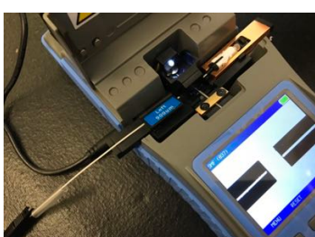
Close bracket over V-grooves
