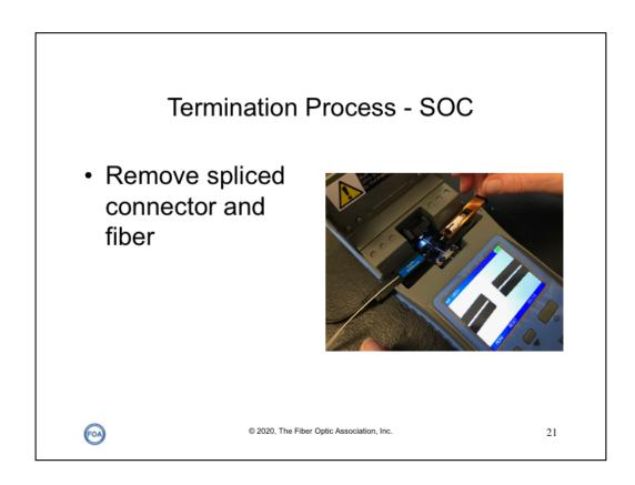
When the splice has been made, remove the spliced assembly from the fusion splicer.
