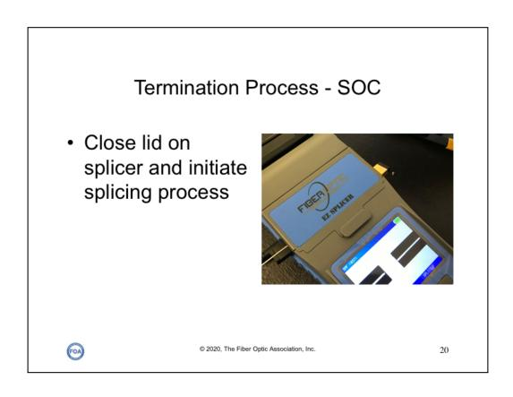
Close the lid on the splicer and initiate the automatic splicing process.
