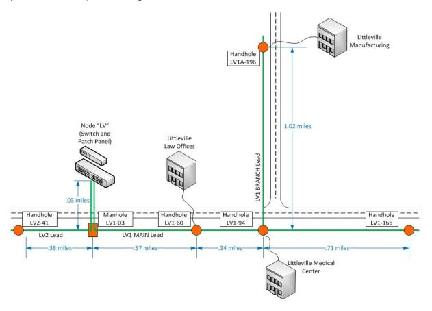
Where a branch is taken off the main lead, we designate that as the "A" lead from LV1, and the remaining numbering convention continues, with the distance is noted in hundredths of a mile.
